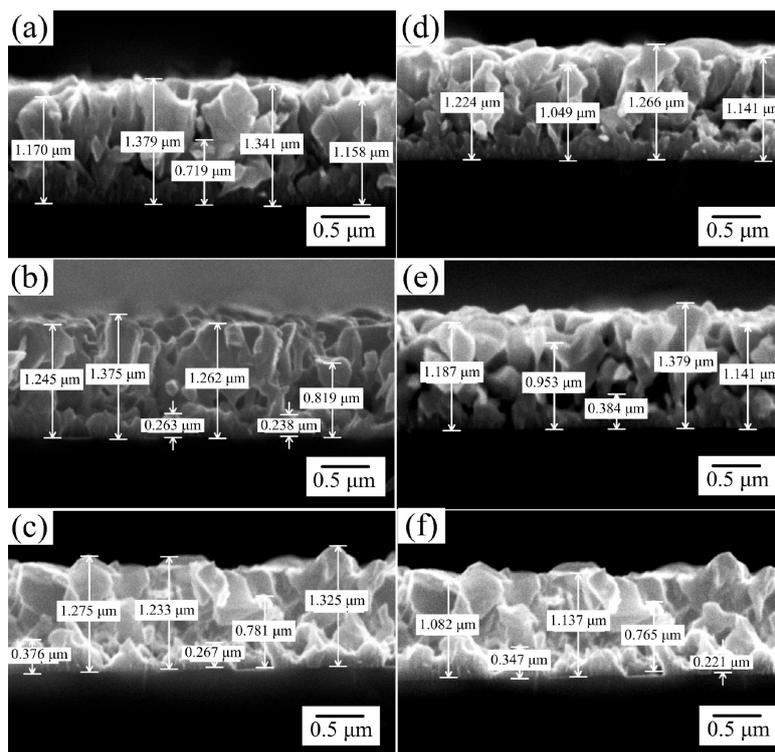
FIGURE 3. SEM cross-sectional images of porous ZnO prepared using  $\text{NH}_4\text{OH}$  solution at (a) 1, (b) 3 and (c) 5 min etching times and using a mixture of 100 mL  $\text{NH}_4\text{OH}$  and 1 mL  $\text{H}_2\text{O}_2$  at (d) 1, (e) 3 and (f) 5 min etching times
