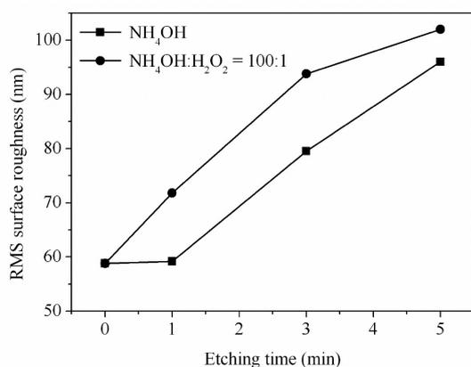
FIGURE 5. Root mean square surface roughness of porous ZnO thin films prepared using  $\text{NH}_4\text{OH}$  solution and a mixture of 100 mL  $\text{NH}_4\text{OH}$  and 1 mL  $\text{H}_2\text{O}_2$  at various etching times
