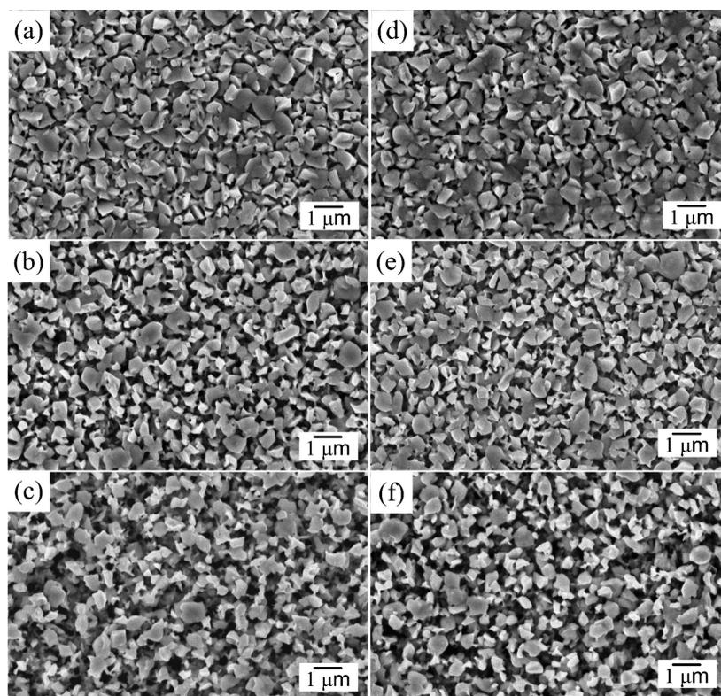
FIGURE 2. SEM images of the porous ZnO surface morphologies prepared using  $\text{NH}_4\text{OH}$  solution at (a) 1, (b) 3 and (c) 5 min etching times and using a mixture of 100 mL  $\text{NH}_4\text{OH}$  and 1 mL  $\text{H}_2\text{O}_2$  at (d) 1, (e) 3 and (f) 5 min etching times
