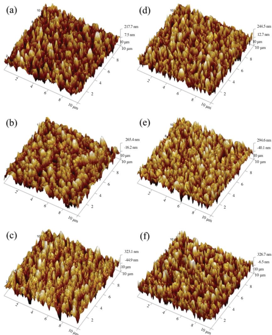
FIGURE 4. AFM topographic images of the porous ZnO thin films prepared using  $\text{NH}_4\text{OH}$  solution at (a) 1, (b) 3 and (c) 5 min etching times and AFM topographic images of porous ZnO prepared using a mixture of 100 mL  $\text{NH}_4\text{OH}$  and 1 mL  $\text{H}_2\text{O}_2$  at (d) 1, (e) 3 and (f) 5 min etching times
