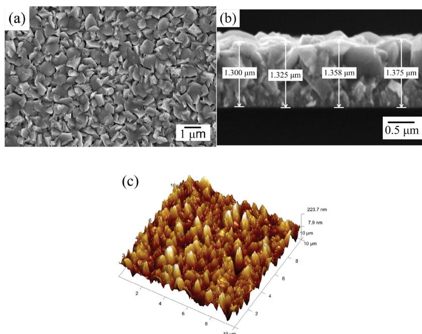
FIGURE 1. Scanning electron microscope (SEM) images of the (a) surface morphology, (b) cross section of the film and (c) atomic force microscope (AFM) topography of as-grown ZnO thin film on n-type Si(111) substrate
